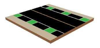
**Curb Extensions** are suitable for when there are no existing parkways and the sidewalk is too narrow to install tree wells.
